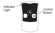
Figure 51 - On/Off Hand-Held Remote Control Unit HRC100
